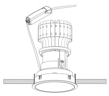
To replace LED module, remove the reflector from the mounting bracket.
