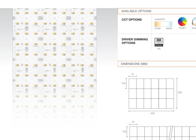
• Width x Length x Height : 300mm x 450mm x 1mm : 300mm x 1800mm x 1mm • Cut Section : 12 LEDs, 100mm x 75mm • LED Pitch : 34mm (L), 31mm (W) 300
